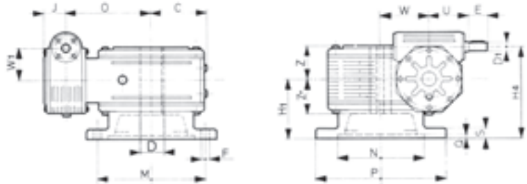
P2 F1 vedi figura - see figura P2 F2 1° rid. albero veloce lato opposto - first reduction high-speed shaft at opposite side
